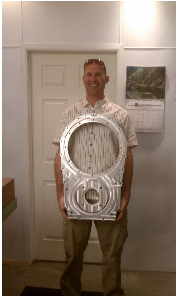
Fig. 3- Actual PSRU case half with Jay Castino of JJC Engineering.
