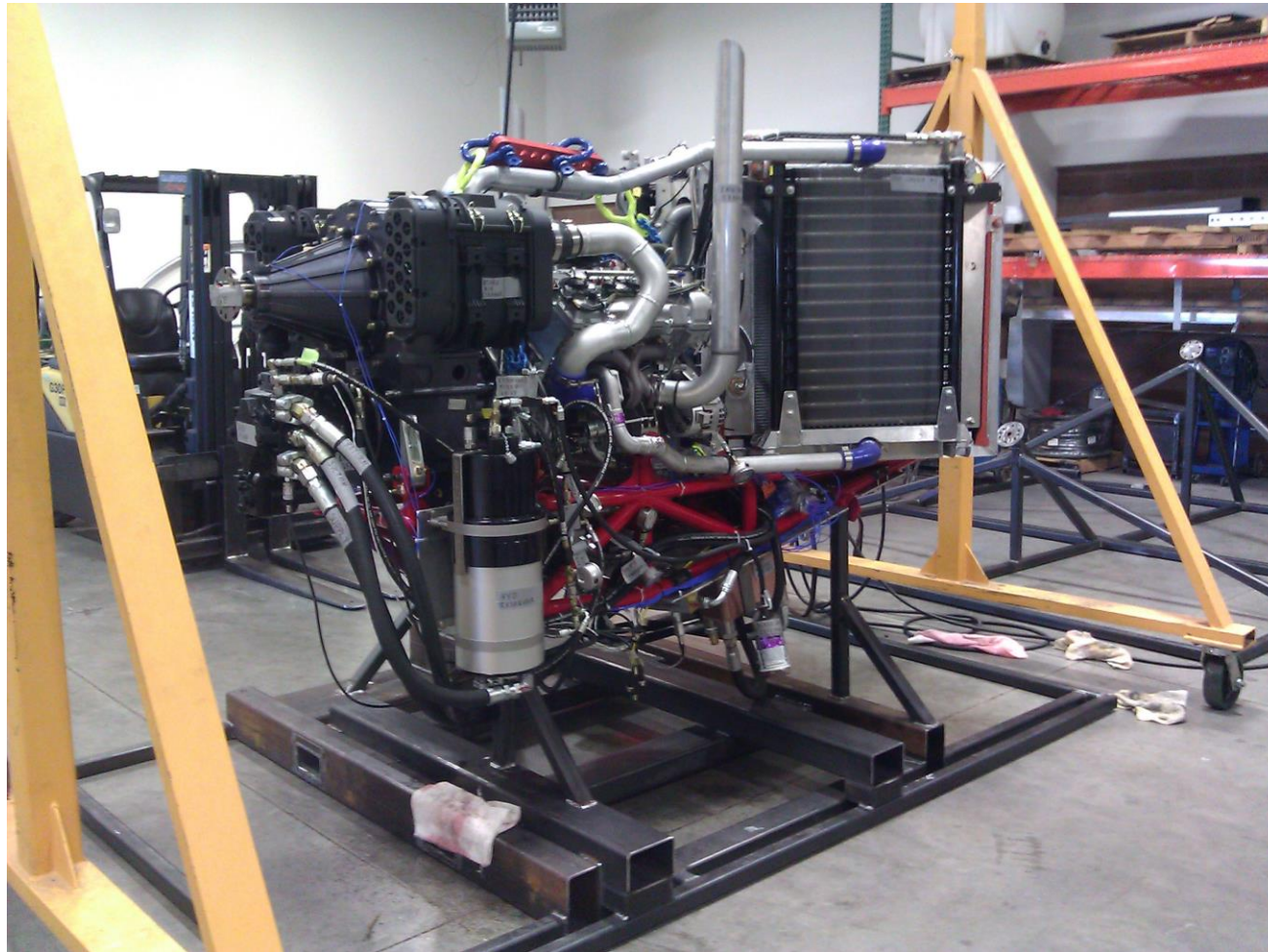
Fig. 4- Loitering engine nacelle test buildup, completed by JJC Engineering and Kawak Aviation.
